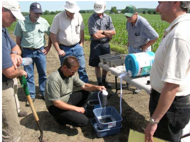
Simulating rainfall to assess a soil's potential for erosion
